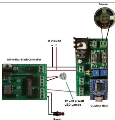
When power is turned on, the Mine Scenario will start to play automatically 1 time. The LED will flash during each explosion.
