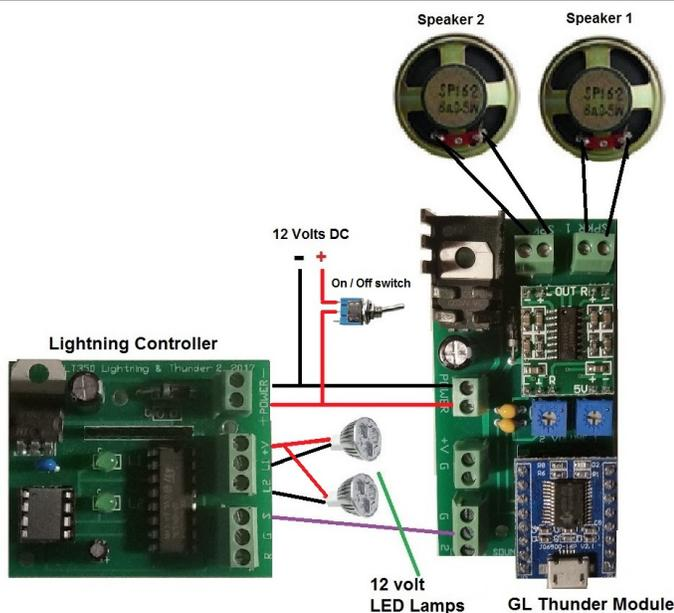
**When** power is turned on, the 2 LED's on the Lightning Controller board will be on and the scenario will have started. In a short time, LED 1, and external LED lamp 1 will flash for about 2 seconds, and shortly after you will hear thunder in speaker one. Then scenario will switch to LED 2, external LED lamp 2 and Speaker 2 back and forth based on the programmed scenario.
